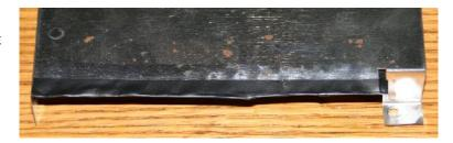
Place strips of tape on the top of the shield, at the back. Approximately nine pieces of tape should be sufficient. Place three pieces of tape beside each other, overlapping somewhat to ensure coverage. Add two more layers, so there's enough thickness built up. You may want to put an additional piece of tape over the edge, too.
