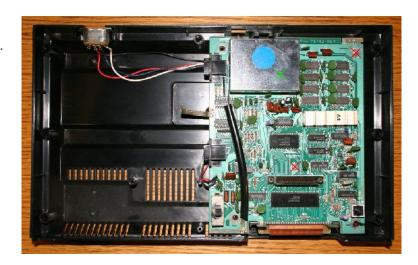
Remove the PCB. These are the parts you'll need to keep. Not shown are the top (with front panel and front expansion door) and bottom of the console.
