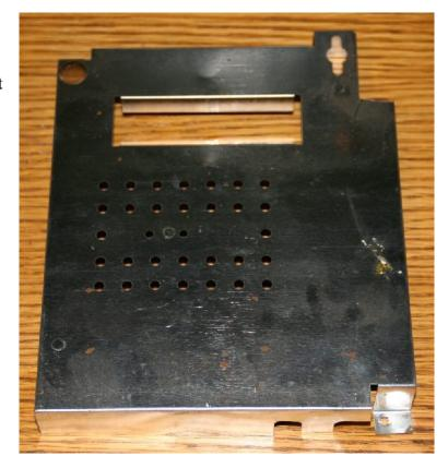
Remove the back part of the shield: with a pair of pliers, gently rock the back flap back and forth until the creased corner breaks free. Be careful not to get cut from the sharp edges. Carefully dispose of the back piece that was removed.
