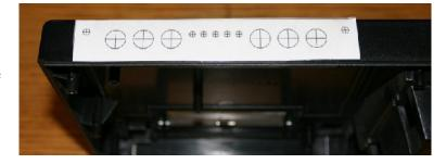
Detail of the taped template. Notice how the bottom edge of the template is flush to the main surface, with no overhang over the lipped edge.
