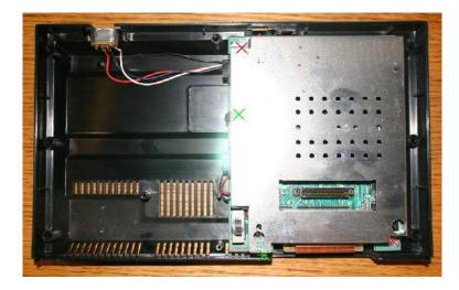
Remove the two remaining screws. Note that all of the twelve screws are the same. Also remove the lid to the modulator.
