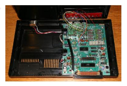
Using a pair of cutters, carefully remove part of the wall of the RF modulator, as shown in the picture. Wear safety glasses when performing this task, and carefully dispose of the extra metal material.
