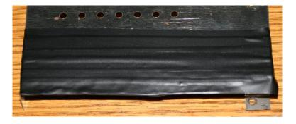
Place the top shield onto the main board.
