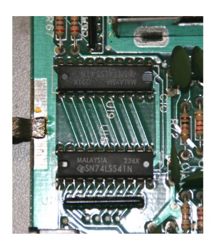
Desolder both chips, and clean up the holes. You could just do the one that has failed, but it's likely simpler just to do both. Make sure all of the traces and pads are in good shape. If they're not, make note of them, so you know which pins require testing and/or repair.
