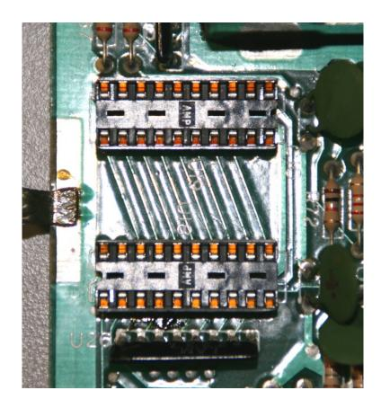
Install 2 new 74LS541 chips. Note the orientation of each chip. As shown in the picture, pin 1 of the top chip is on the upper right, and pin 1 of the bottom chip is on the lower left.
